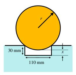
The diagram shows a ball of radius, r, 73 mm rolling along a groove of width 110 mm and depth 30 mm. Calculate the length marked x.
